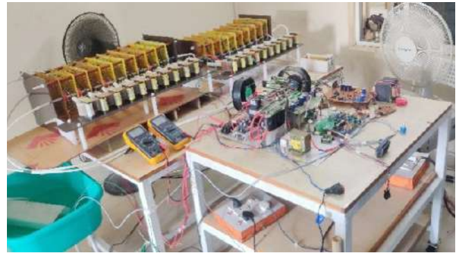
Figure B.11 Prototype high voltage power supply for Gyrotron body circuit through local industry
