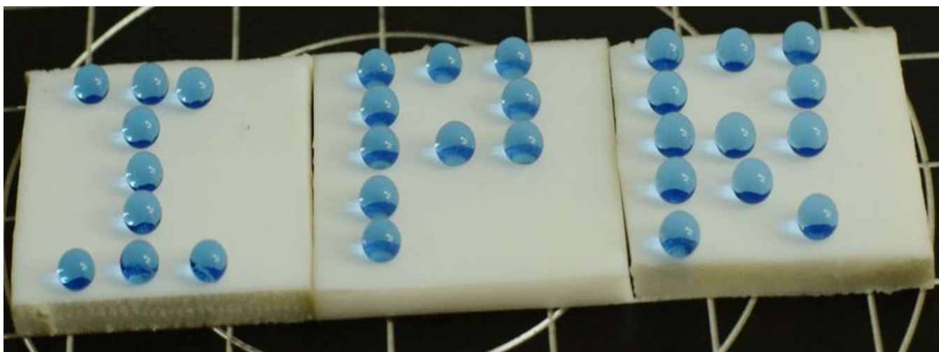
Figure A.1.1 Photograph of the Hydrophobic PTFE surface produced
