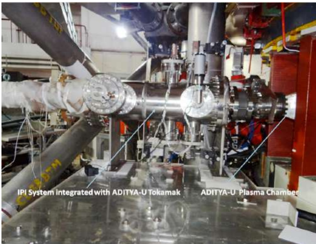
Figure A.3.1.2 – Electromagnet Pellet Injector integrated to the Aditya-U tokamak
