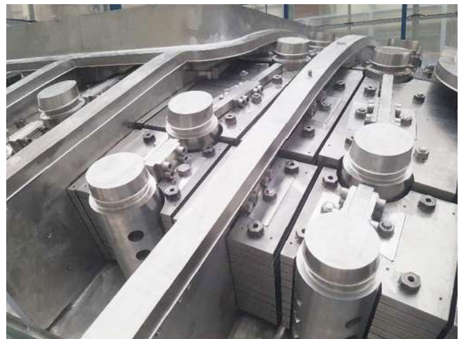
Figure B.5 Installation of IWS blocks in vessel section at Korean domestic agency
