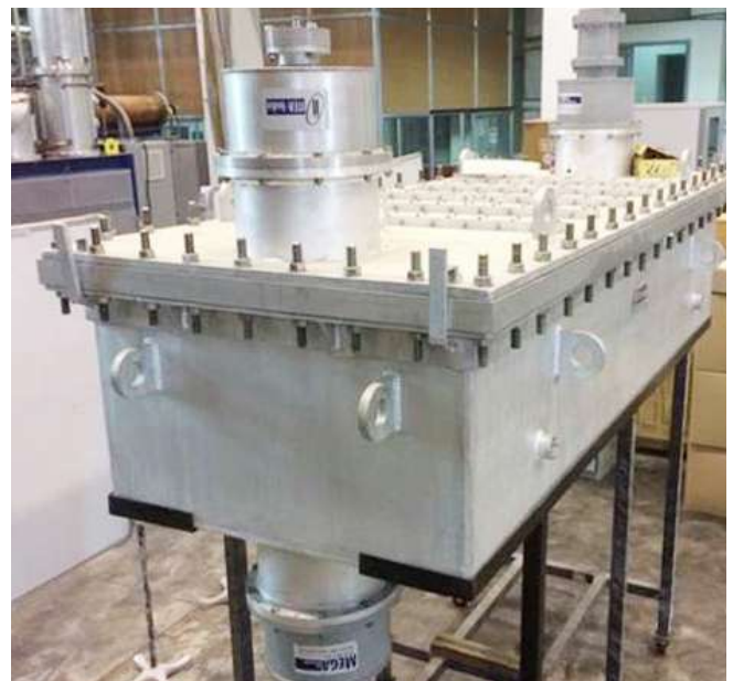
Figure B.10 A New type of wide-band Hybrid Mega-Watt level Continuous Wave Radio Frequency Combiner / Splitter
