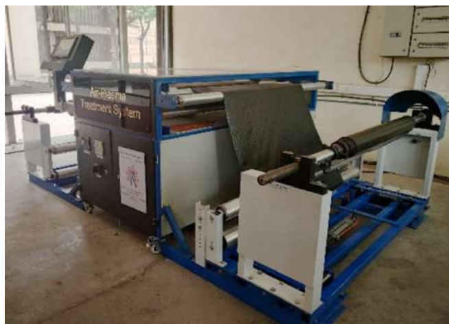
Figure A.1.2 Air-plasma treatment system installed at CIPET
