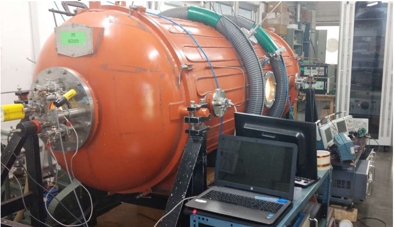
Figure A.2.6 The experimental device to study the Whistler waves.
