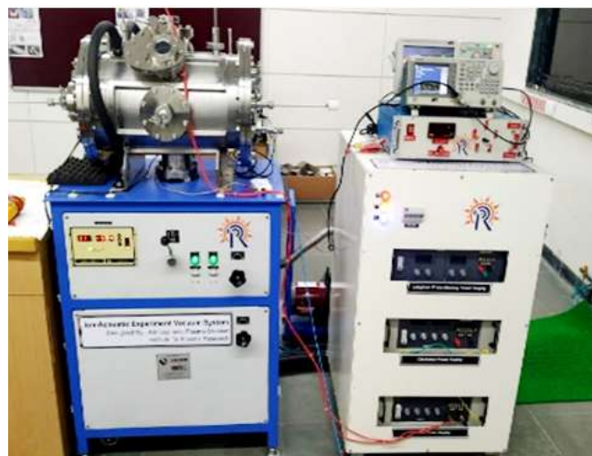
Figure A.1.3 Ion-Acoustic Wave and Langmuir Probe System installed at UM-DAE CEBS
