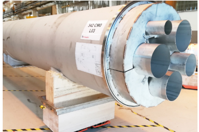
Figure B.3 Cryoline elements, having one of the biggest diameters (DN1000 and locally increases to ~1320mm) under manufacturing at factory
