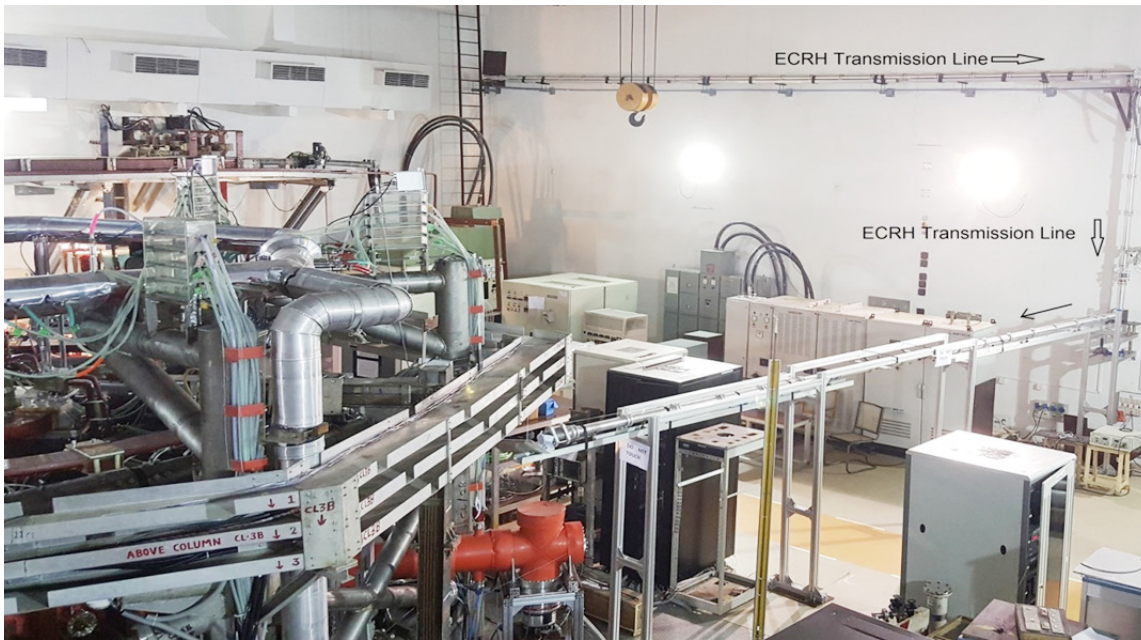
Figure A.3.3 ~75meter long transmission line is used to launch ECRH power from SST- hall to ADITYA-U tokamak, consisting of 63.5mm ID corrugated waveguide, bends, polarizer, DC breaks & bellows etc
