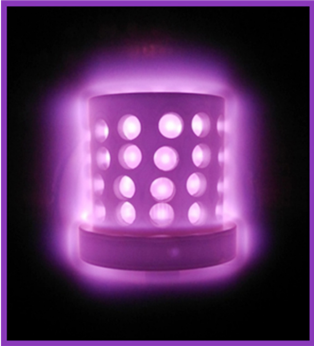
Figure A.2.1 Active screen plasma nitriding
