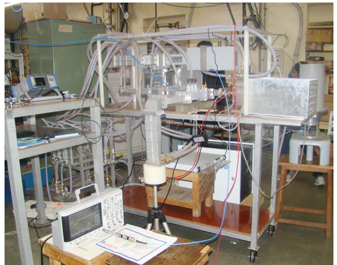
Figure A.1.3 Magnetron system, integrated with the pulsed modulator and the HPM coupling components.
