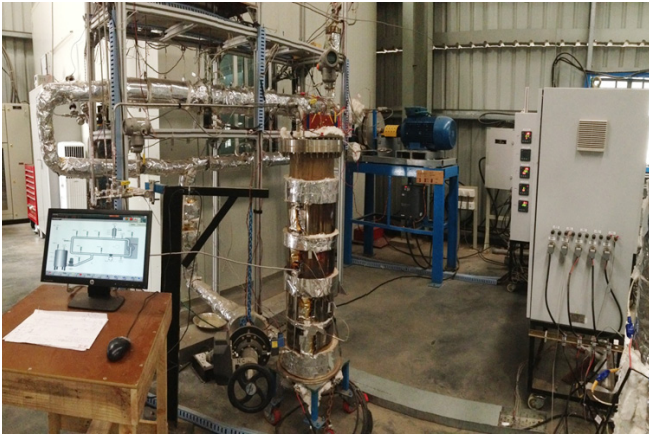
Figure A.2.6 Panoramic view of the Lead-Lithium (Pb-Li) heat transfer experimental loop
