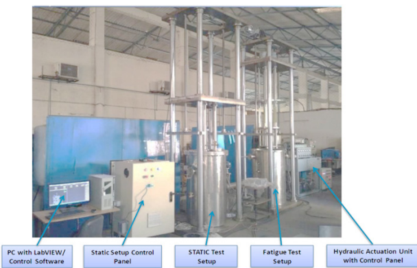
Figure A.2.1 Integrated MCFLT at factory site
