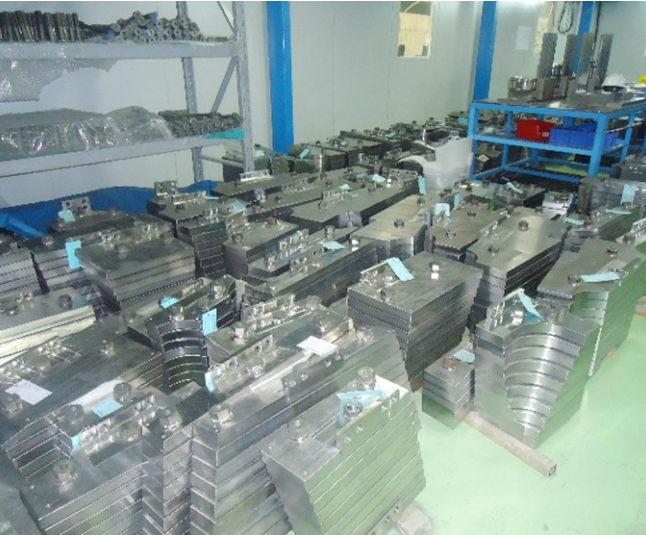
Figure B.1 In-Wall Shielding Block Assemblies – manufactured and being readied for testing
