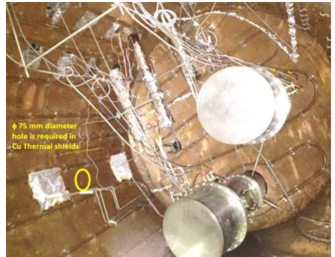
Figure A.1.12 Inside View of current Feeder System
