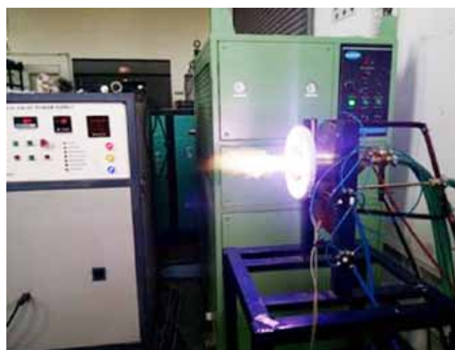
Figure A.3.13.1 atmospheric pressure non-transferred dc plasma torch operating at \sim 50 kW, along with power supply and heat exchanger
