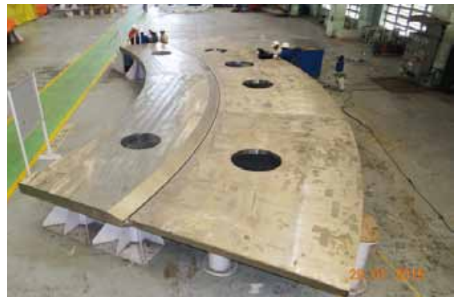
Figure B.2.2 Cryostat Base Section Tier -2 – fabrication in advanced stage
