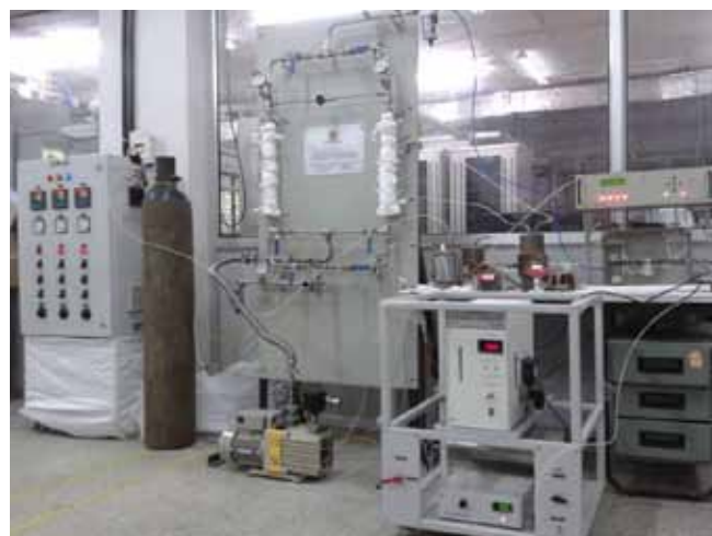
Figure A.2.9.1 Atmospheric Molecular Sieve Bed system under operation
