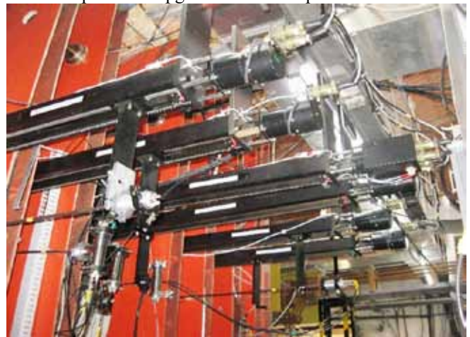
Figure A.3.1.3 A few large, linear motion, vacuum interfaced probe drives with \sim 1\text{ m} travel length
