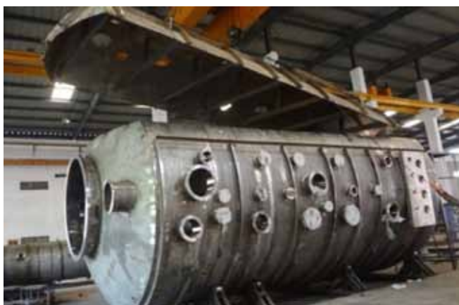
Figure A.2.7.3 Manufacturing of Indian Test Facility Vacuum Vessel
