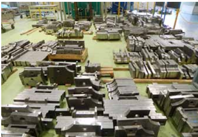
Figure B.2.1 In-Wall Shielding manufactured blocks
