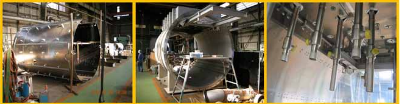
TACB thermal shield, TACB Outer Vacuum Jacket & TACB Top Plate with Cryogenic Valve Body inserted
