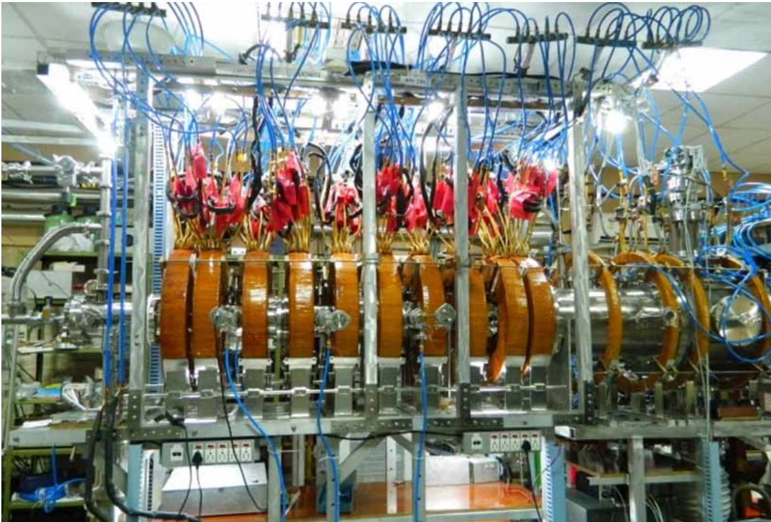
Figure A.3.6.1 Picture of Inverse Mirror Plasma Experimental Device (IMPED) set up at basic plasma laboratory
