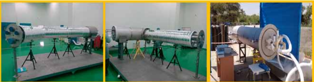
Manufacturing of Prototype Cryoline @ INOX CVA, Testing of Prototype segment is under progress
