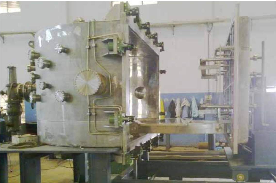
Figure A.2.2.1 D-shaped double walled vacuum chamber & target handling system for testing components whose weight is up to 1 tonne
