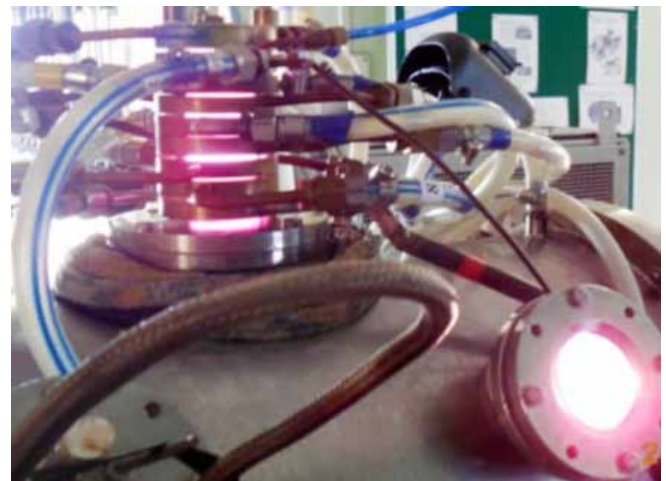
Figure B.3.2 Tungsten samples are being exposed to Helium plasma
