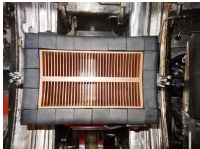
Figure A.1.2.5 Photograph shows the installed LHCD antenna system on SST-1 machine when viewed from inside the machine. The probe-hats housing electrical probes are also seen on either side of the antenna.
