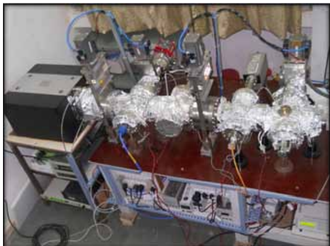
Figure A.2.3.1 Out-Gassing Measurement system
