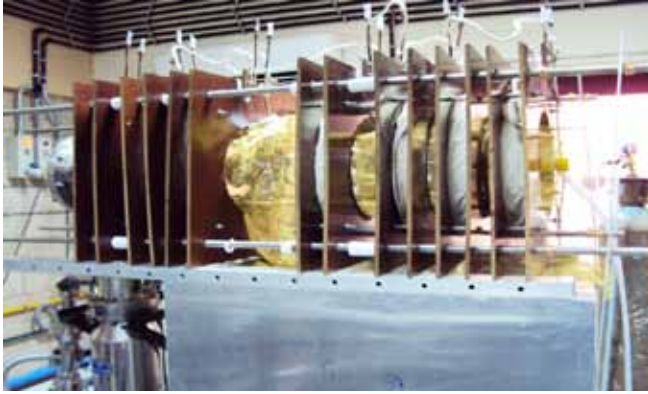
Figure A.3.10.1 Experimental set-up of the linear Helicon plasma device
