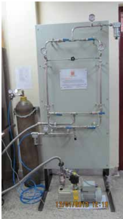
Figure A.2.10.1 Picture of the fabricated PSA system
