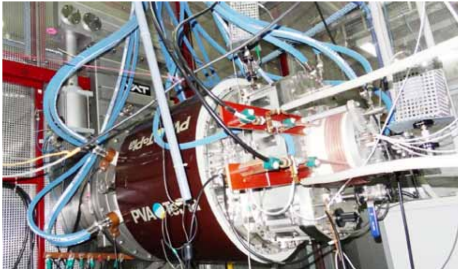
Figure A.2.7.1. Negative ion source test bed, ROBIN, with assembled extraction system
