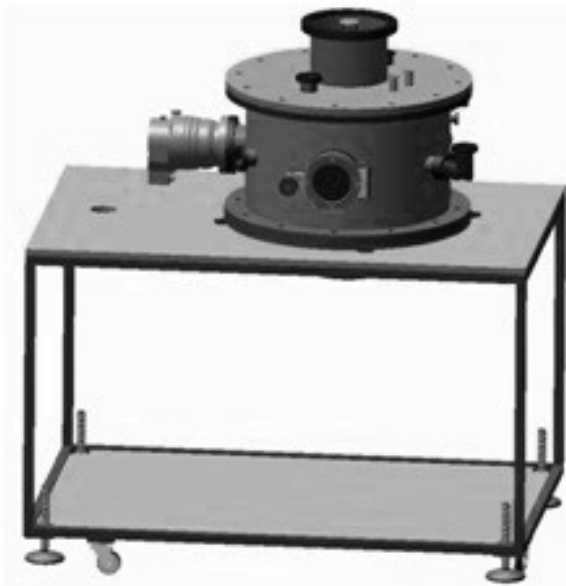
Figure B.3.2 Drawing of cylindrical inertial electrostatic confinement fusion (IECF) chamber
