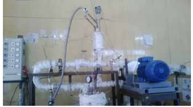
Figure A.2.4.3. Lead-Lithium loop for testing loop diagnostics
