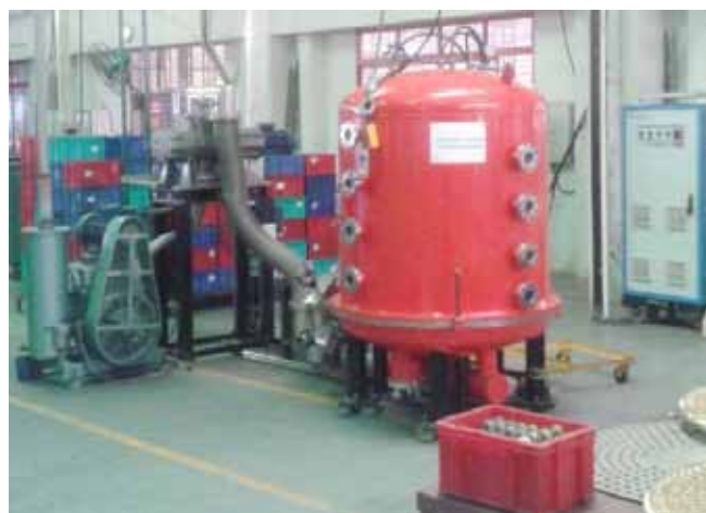
Figure B.1.4 Photograph showing the installed plasma surface modification system
