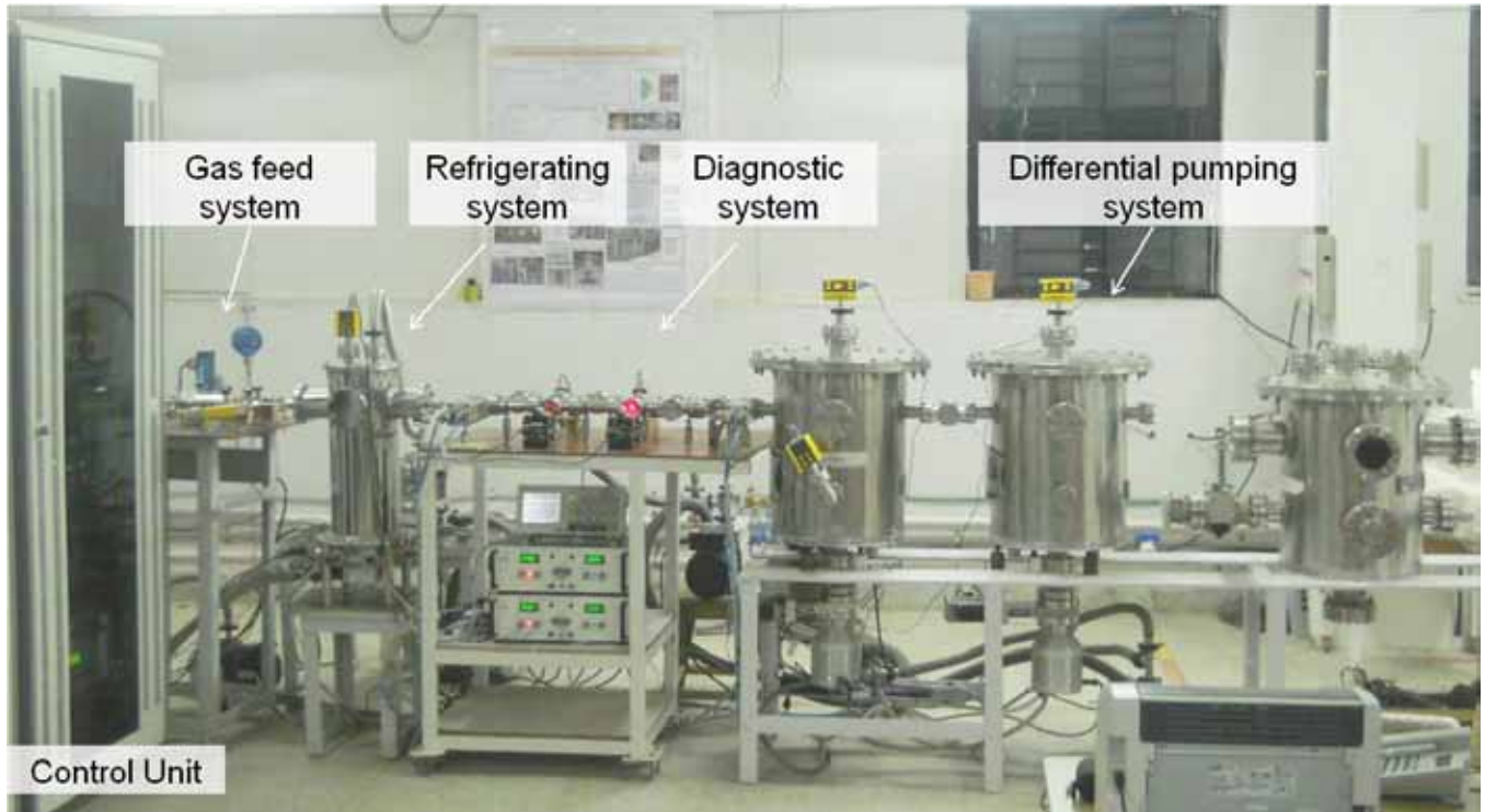
Figure A.2.3.3 Single Pellet INjector System (SPINS)
