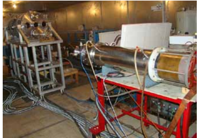
Figure A.3.4.1 the VIRCATOR and the plasma systems prior to coupling
