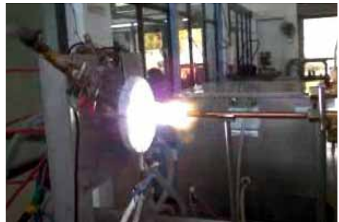
Figure B.1.1.2 : Photograph of the torch in operation along with enthalpy probe
