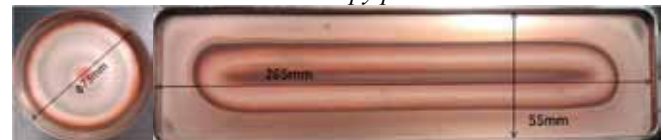
Figure B.1.1.3 : Photographs of (a) circular and (b) rectangular magnetron cathodes (targets)
