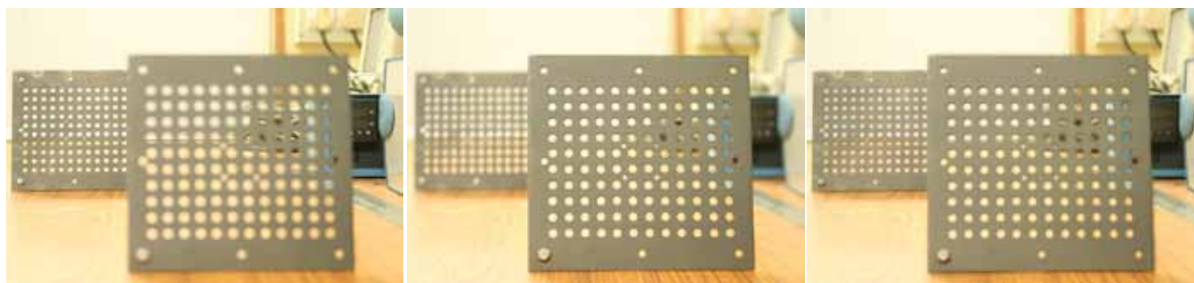
Figure A.1.1.2.1 Figure A.1.2.2.2 Fusion of visible images out of focus. (a) Visible image with focus on back object. (b) Visible image with focus on front object. (c) Fused image with uniform focus.
