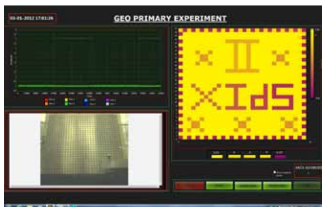
Figure B.1.4.1 : By using a non-contact electrostatic probe, intensity charge displaying the potential distribution over the surface of printed circuit board depicting the satellite solar array dimension
